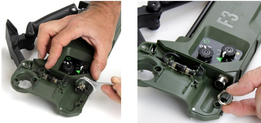
Figure 32: Removing the Coil Connector Nut (18mm)
