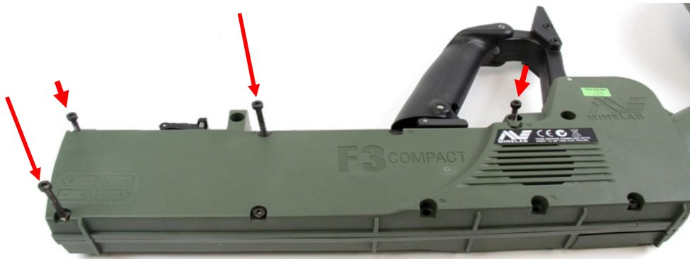
Figure 23: Fitting Four Screws
