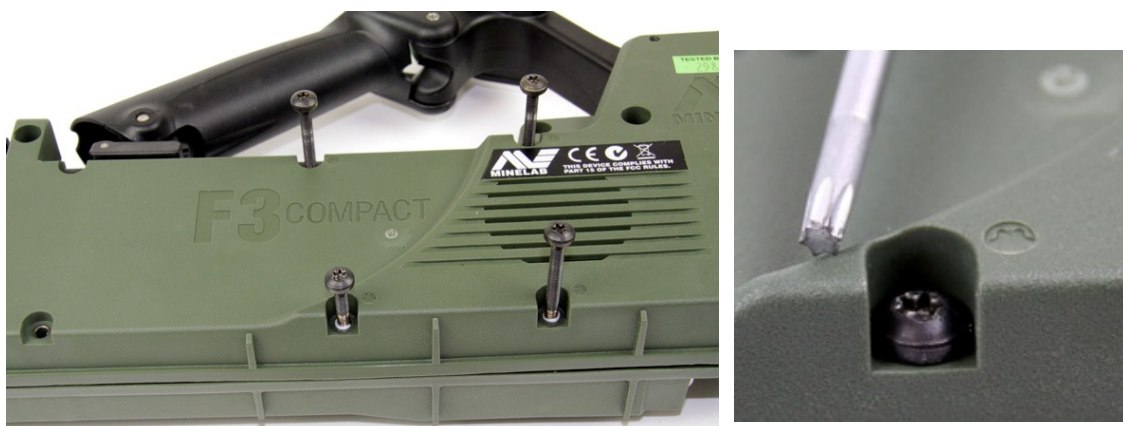
Figure 13: Removing Four Torx Screws
