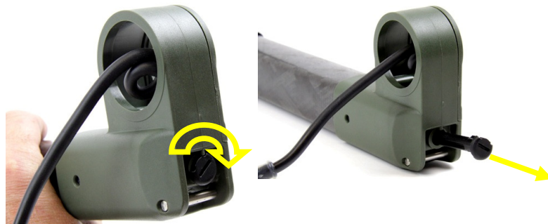
Figure 51: Removing Pin Coil Cable
