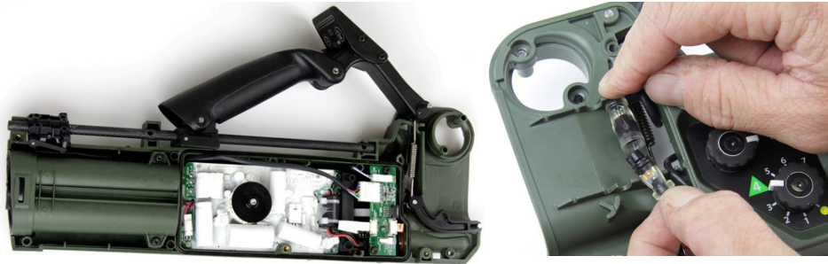
Figure 80: Disconnect Wiring Loom Handle
