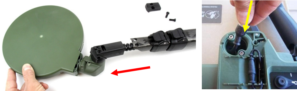
Figure 53: Sliding the Coil Off the Shaft
