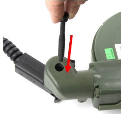
Figure 63: Inserting Pin Coil Pivot
