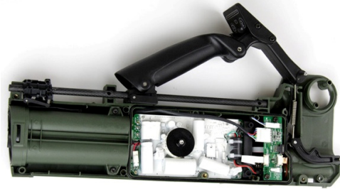
Figure 89: Opened Detector Body
