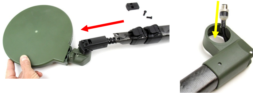
Figure 77: Removing Coil Cable from Shafts
