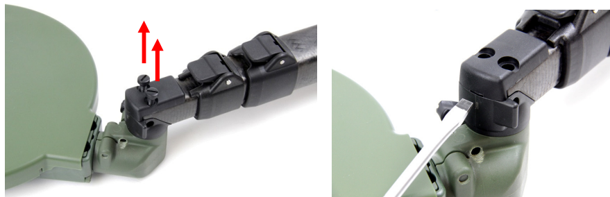
Figure 76: Removing Screws from Lower Shaft
