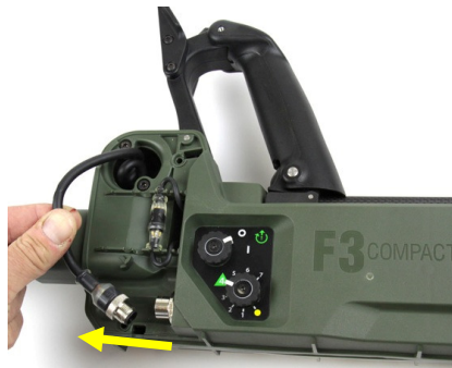
Figure 50: Disconnecting Coil Connector
