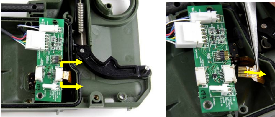
Figure 92: Disconnecting Six Way Ribbon Cable
