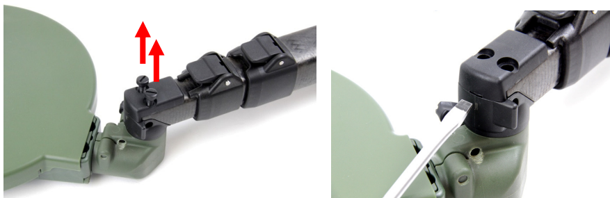
Figure 52: Removing Screws from Lower Shaft
