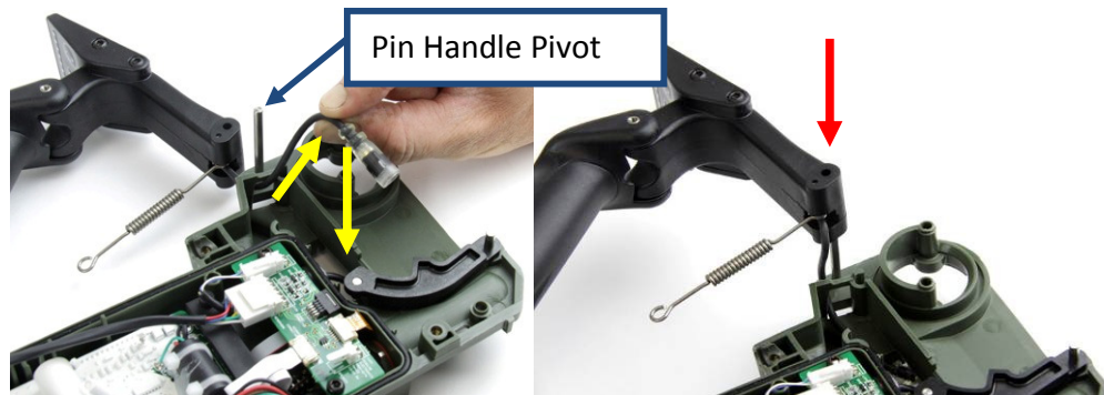
Figure 83: Threading the Wiring Loom
