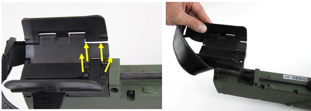
Figure 9: Removing the Armrest
