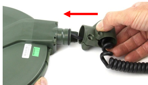
Figure 61: Fitting Pivot Coil Yoke
