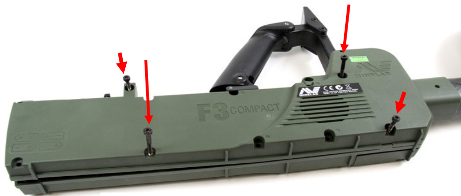
Figure 22: Fitting Four Screws
