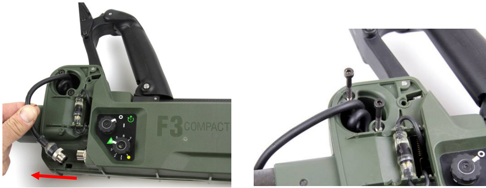
Figure 11: Disconnecting Coil Plug and Removing Screws
