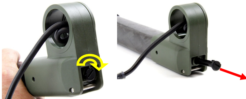
Figure 75: Removing Pin Coil Cable
