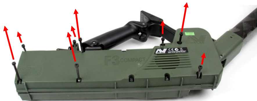
Figure 12: Removing Eight Screws (Allen Key)
